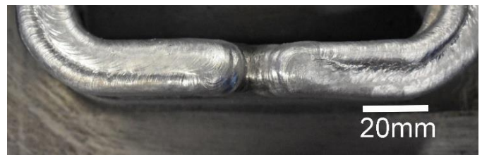
Figure 18: Inner and outer bead sagging, top view
