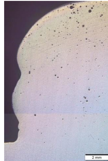
Figure 11: Block utilizing torch oscillation with improved inter-bead and toe fusion, reduced fairness
