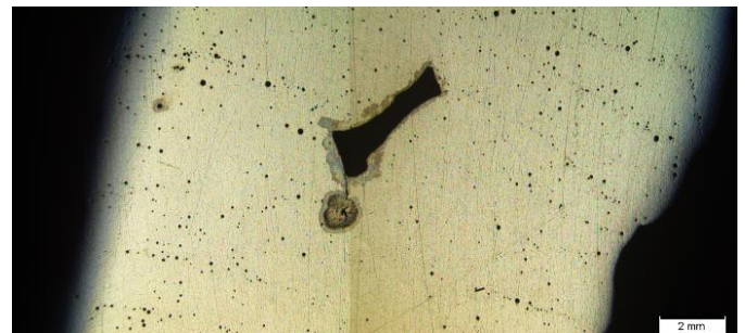
Figure 22: Macrosection of thin-wall circular build, inter-bead void and inter-layer porosity visible
