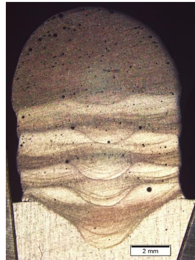
Figure 5: Cross-section of wall build, etched, showing poor toe fusion but good inter-layer fusion and acceptable fairness
