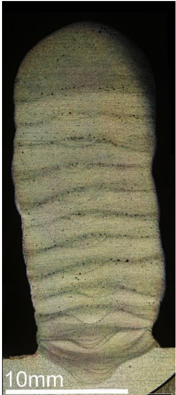
Figure 12: Wall utilizing 2.5 Hz torch oscillation, etched, with excellent toe fusion. Vertical fairness needs improvement through additional parameter refinement.
